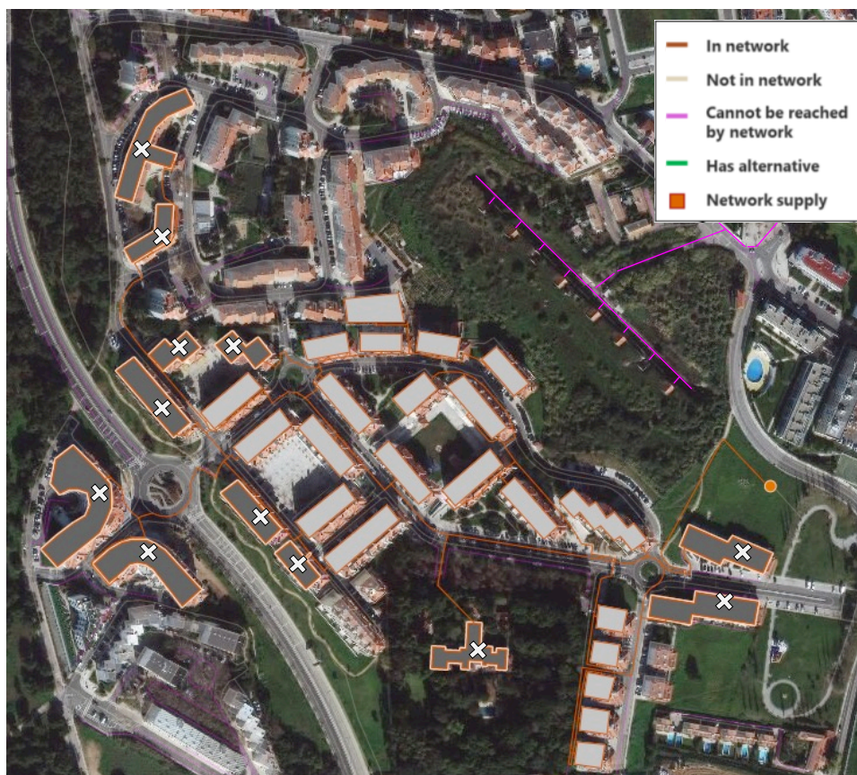
Figure 6-5. Solution network – Optional building included (in dark grey)
