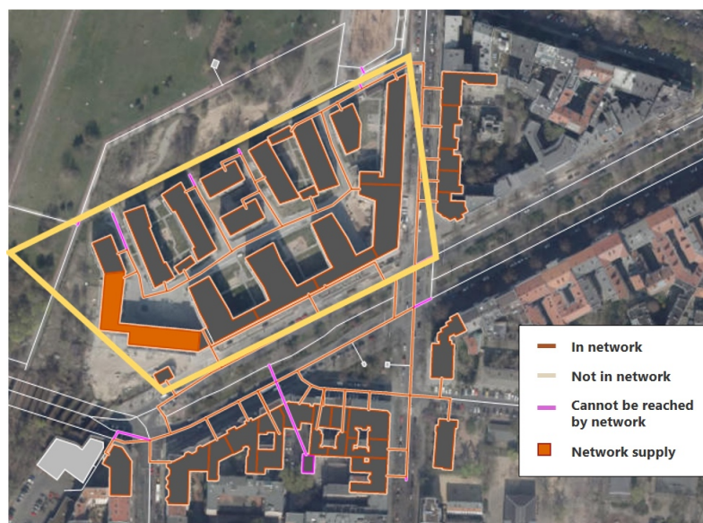
Figure 3-3. Solution presentation of the new district connected with neighbouring old district (yellow shaped existing district heating supply area)
