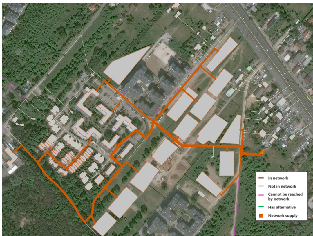
Figure 5-4. Area n° 1 network topology solutions 1-3
